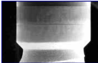
Figure 1. (A) Scanning electron micrograph (SEM) of the surface of a laser microtextured implant. The microtexturing is in two bands on the two millimeter-wide collar. (B) Higher magnification SEM of the laser microtextured surface showing 12µm grooves and ridges (bar = 40µm).
