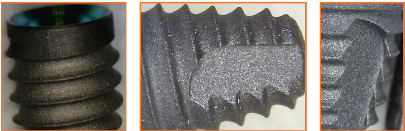
Figure 19. No evidence of surface abrasions on the BioHorizons implant samples. There is a notable change in coloring between the implant collar and the implant body due to the Laser-Lok application around the collar.
