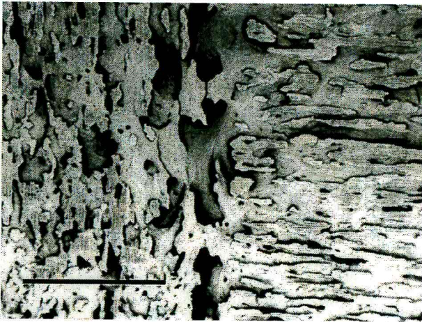
Figure 17. Low power scanning electron micrograph of a deproteinated bone specimen from the IM rod study. The implant has been removed, and many small areas of bone attachment to the surfaces are seen. The bone is oriented according to the microgrooving on the implant, which was oriented longitudinally (horizontal) on the right segment and circumferential on the left segment. A 300 \mu\text{m} seam with no microtexturing was in the center. Bar = 1000 \mu\text{m} .
