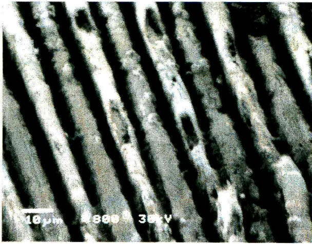
Figure 20. High power scanning electron micrograph of a deproteinated bone specimen from the IM rod study. The implant has been removed exposing ridges of bone mineral that had been in the microgrooves of the implant. Oriented openings left by cells are visible in the mineral structure.
